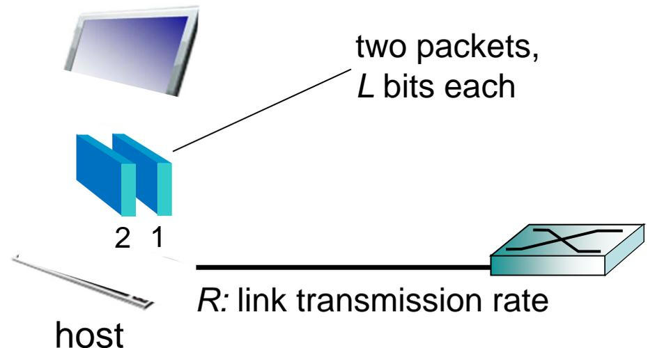
$$\text{packet transmission delay} = \text{time needed to transmit } L\text{-bit packet into link} = \frac{L \text{ (bits)}}{R \text{ (bits/sec)}}$$
