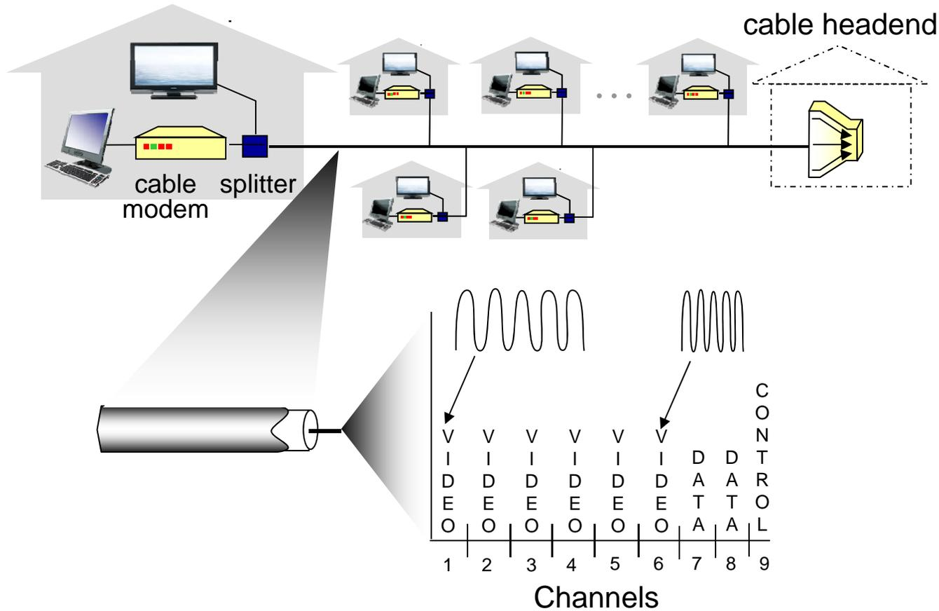
***frequency division multiplexing:*** different channels transmitted in different frequency bands
